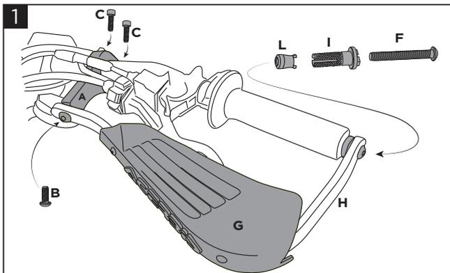
**1** Assemble the cover (G) on the bar (H). Insert the screw (F) through the bar (H) and screw the expander (I) with the insert (L) without tightening. Assemble the bracket (A) to the bar (H) using the screw (B) and tighten. Insert the handguard assembled on the handlebar, tighten the screw (F) and fix the collar of the bracket (A) using the screw (C).
